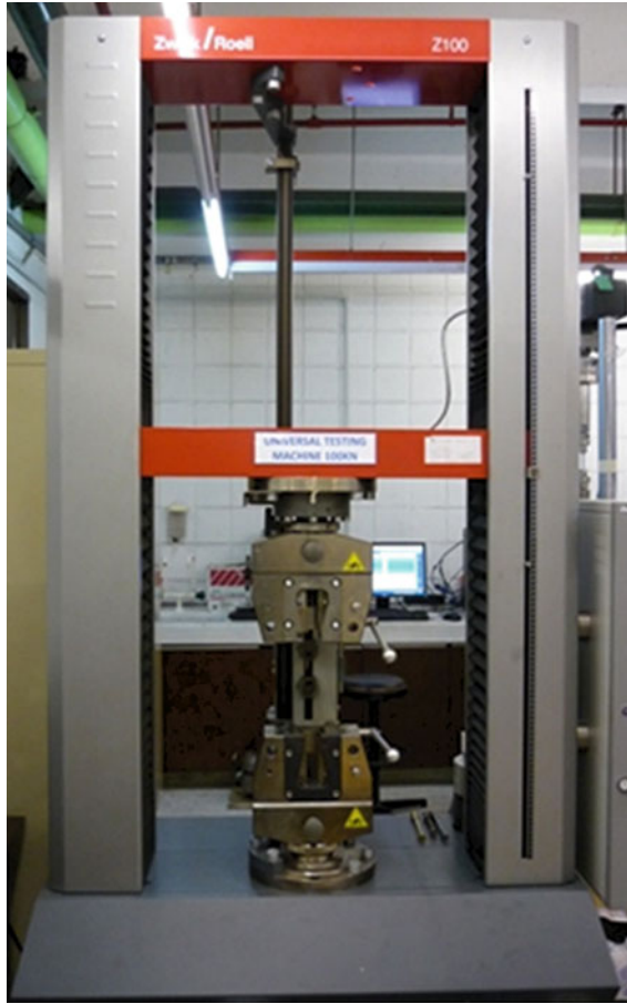
Fig. 4 Universal testing machine with a capacity of 100 kN
